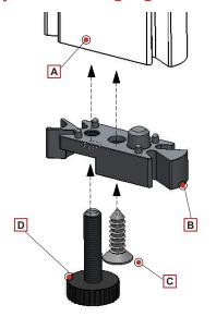
A x 1 Slim 3m metal profile **B** x 1 Metal intermediate foot C Self-tapping screws Ø5.5 D Adjustable Leveling Leg
