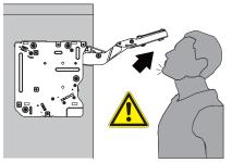
The Arm of this device could spring up and cause injury. Do not push the arm down with door properly attached
