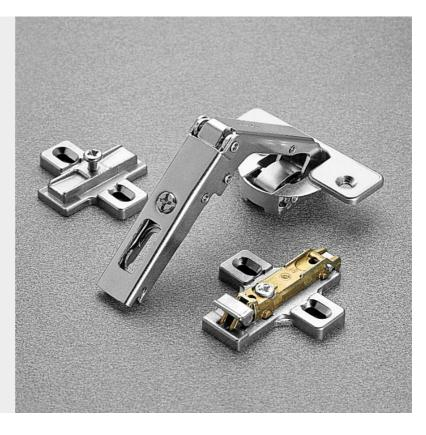
Hinges for corner cabinets. 11 mm deep die-cast cup. 35 mm cup diameter. Opening angle of the first door 70°. Possible drilling distance on the door (K): from 3 to 6 mm.
