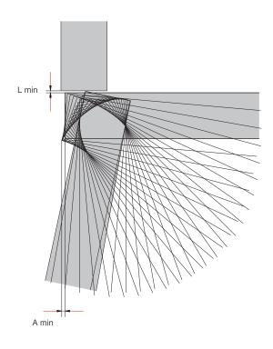
Simulation of the Opening of a 110 Degree Full Overlay Door
