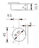
Use these formulas to determine the type of hinge arm, the drilling distance "K" and the height of the mounting plate "H" for each door application
