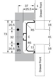
Suggested reveal between drawer fronts is 41mm. Minimum suggested between fronts is 30mm. Suggested overlap is 11mm for comfortable grip.
