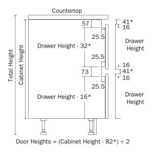
\* Recommendation based upon two equal drawers. Adjust accordingly. Minimum Gap Suggested 30mm.
