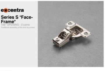
Stamped steel. Cup depth 11 mm (7/16'). Opening 106' degrees. Drilling distance (K) fixed at 2.5 mm (3/32'). Gap between door and frame (L) = 4.6 mm.
