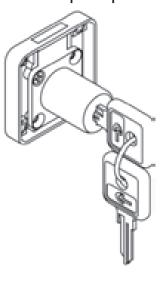
▶ 1&2 Install cylinder core with key inserted into the cylinder housing. Be sure to align the two diamond shaped objects on both the cylinder core and the cylinder housing.
