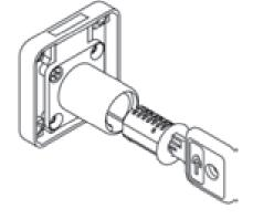
**▶ 1&2** Insert removal key into cylinder core.
