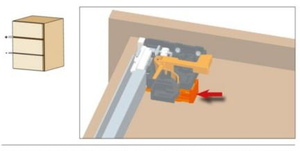
Push the lever towards the outside of the drawer to achieve the height adjustment. This operation is tool free.
