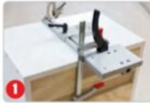
1 Clamp jig in desired location.
