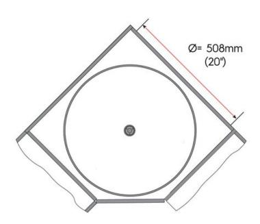
Mechanism Height 533-838 mm (21" - 33")
